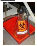
These liquids must be stored in closed, leakproof containers while awaiting treatment and disposal. Collection vessels should be secured so that they cannot be tipped over. Secondary containment is strongly recommended and can be achieved by placing the vessel in a bucket or deep tray.
